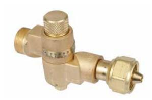
Model BHA 2 adjustable head adds flexibility to machine cutting torches by allowing bevel cuts without changing the position of the torch. It can be set at any angle from 0 to  $90^{\circ}$  on either side of vertical.
