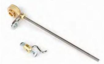
Circle Cutting Attachment is easily attached to a cutting torch or cutting attachment. The roller guide is adjustable to various heights and is designed to hold the cutting tip at exact pre-set distance from the work. Cutting range 1.5" (38.1 mm) - 28" (71.1 cm) circle.
