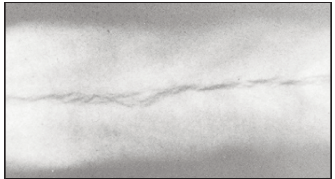
Figure 11: Radiograph Showing Longitudinal Weld Cracking
